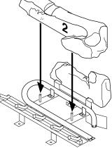
Figure 54 - Installing Log No. 1
